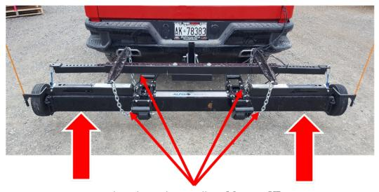
4 chains loose when travelling. Magnet is UP. Higher travel speeds (greater then 10mph/16kph)
